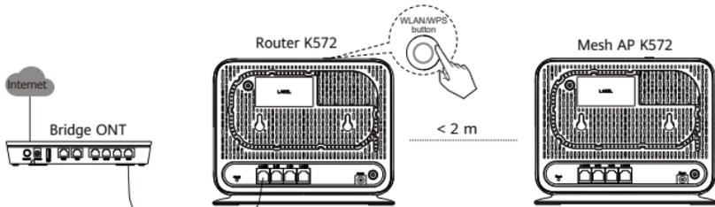
Wait until the mesh AP K572 indicator turns steady white, which indicates that the pairing is successful.
