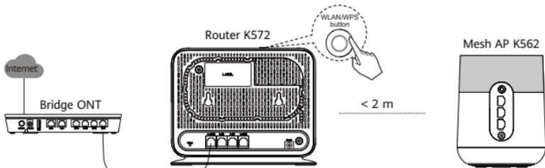
5 Wait until the K562 indicator turns steady white, which indicates that the pairing is successful.
