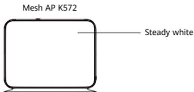
7 Unplug and move the mesh AP K572 to the position where the Wi-Fi coverage is to be expanded. Then power on this K572.
